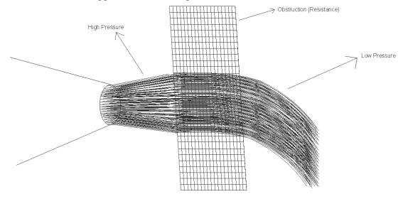
Here, on the incoming side, there is a higher pressure (potential) and at the outgoing side of obstruction (resistance), there is a lower pressure (potential). There is a fall of pressure (potential) across the mesh (resistance).
